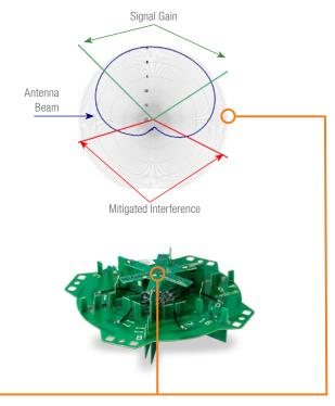
BeamFlex not only focuses RF energy only where it's needed but also mitigates interference coming from other directions. This ensures that the highest possible PHY rate is used and that the highest possible throughput is achieved for all clients.
